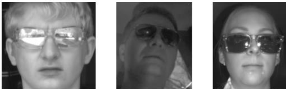
Figure 4: These are images where Guardian cannot track and see the eyes because lens transmissivity less than 50%
